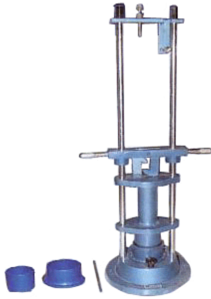
Sample subjecting to hammer blows
