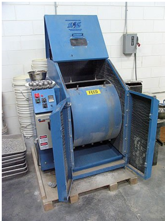
L.A. abrasion testing equipment
