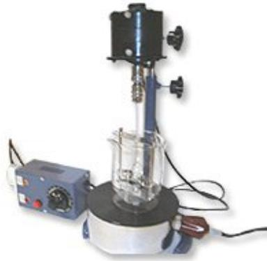
Softening point test for bitumen.
